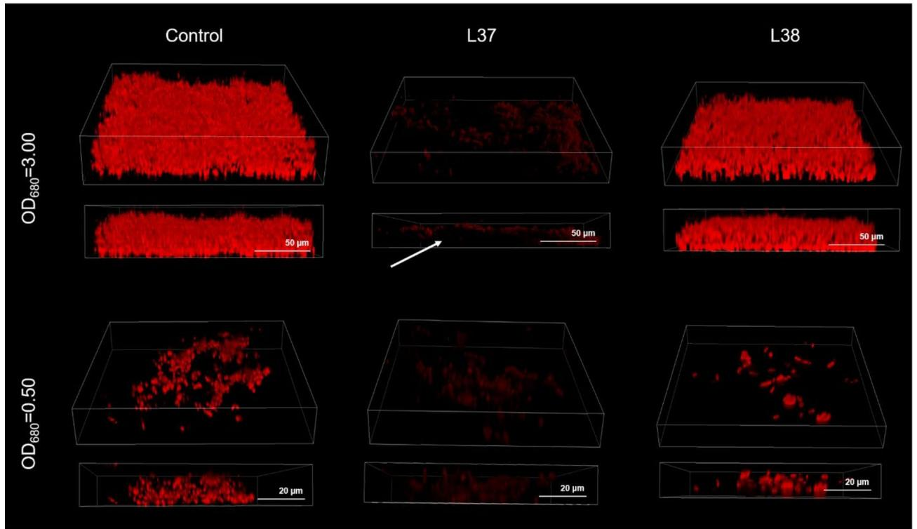
**Fig. 4.** The 3D CLSM micro images of algal biofilms in cross-section after growing for 14 days on a wood substrate coated with the most and least effective polysiloxane compounds; the arrow highlights the absence of autofluorescence in the high-density biofilm in contact with the surface of the wood treated with L37; scale bar 50  $\mu\text{m}$  and 20  $\mu\text{m}$ .
