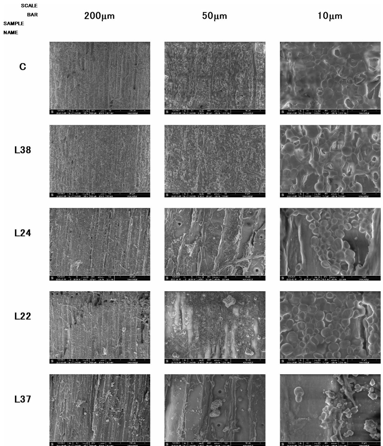
**Fig. 6.** SEM photomicrographs of microalgal biofilms after 14 days of growth on wood: Control (C), L38, L24, L22, L37 coating. Scale bar: 200  $\mu$ m, 50  $\mu$ m and 10  $\mu$ m.
