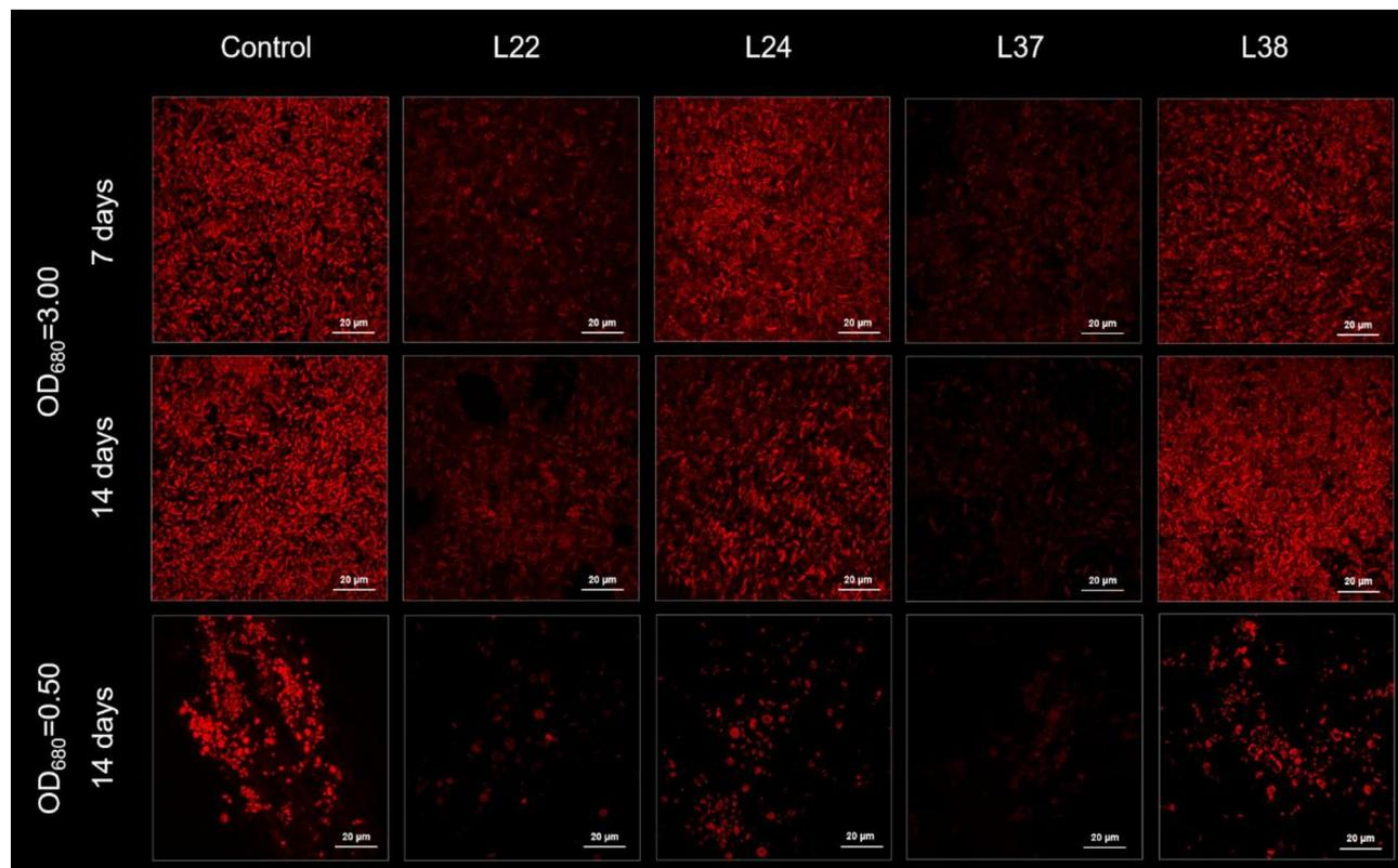
**Fig. 3.** The CLSM micro images of chlorophyll fluorescence in algal biofilms growing on a wood substrate coated with polysiloxane compounds; scale bar 20  $\mu\text{m}$ .
