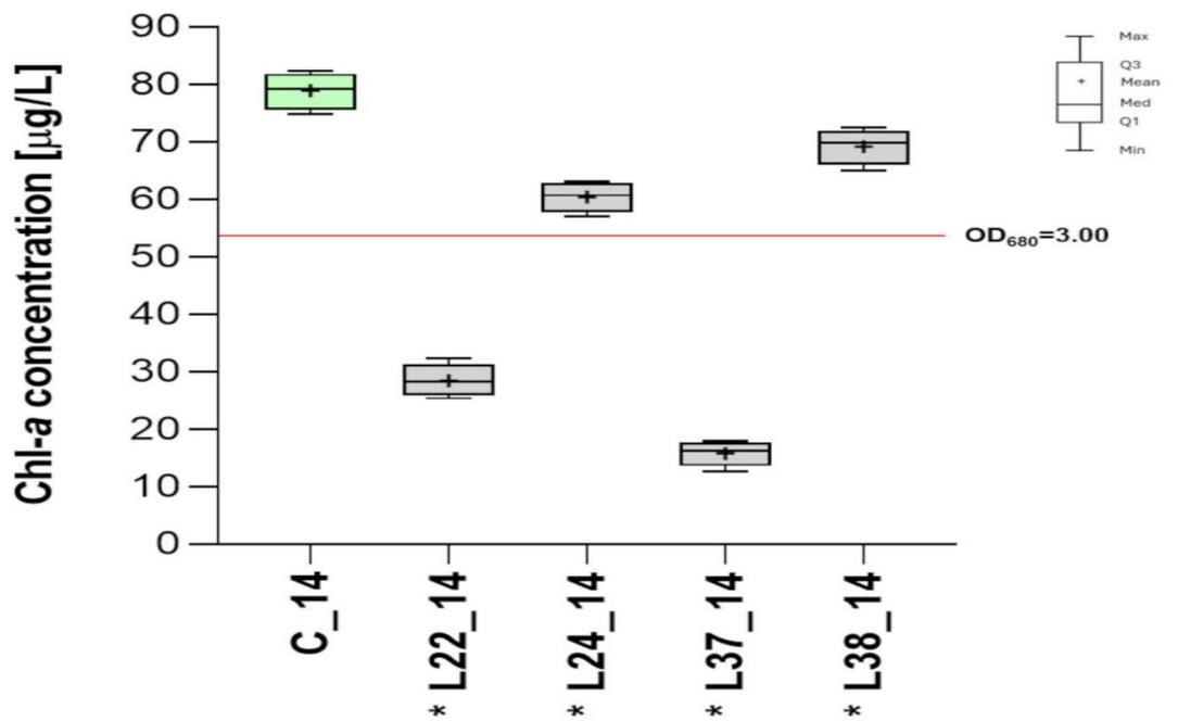
**Fig. 5.** Changes in the chl-*a* concentration of the microalgal biofilm for the control wood substrate and the samples coated with polysiloxane compounds after 14 days of cultivation; black asterisks indicate the statistical significance ( $p \leq 0.05$ ) of the differences between the samples and the control, while the solid red line shows the chl-*a* concentration of the inoculation mixture.
