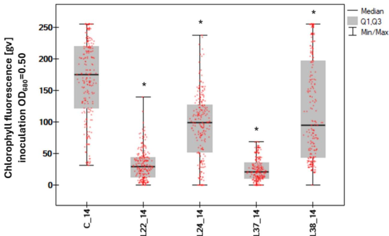
**Fig. 2.** Changes in the  $^{chl}FI$  of microalgal cells ( $OD_{680} = 0.50$ ) on a plain wood substrate (control) and wood substrates coated with polysiloxane compounds (treated samples) after 14 days of cultivation; the black asterisks indicate the statistical significance ( $p \leq 0.05$ ) of the differences between the treated samples and the control.
