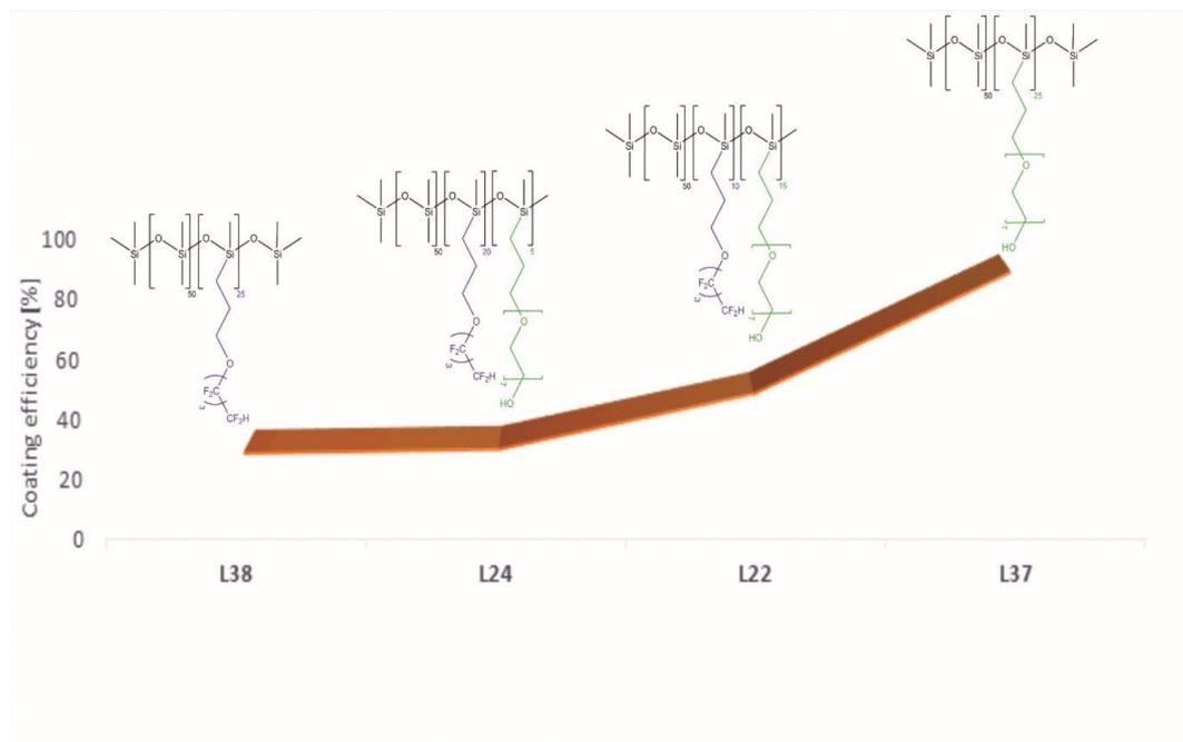
**Fig. 7.** Curve of the effect of the number and type of functional groups in the polysiloxane on the biological properties of the coating.
